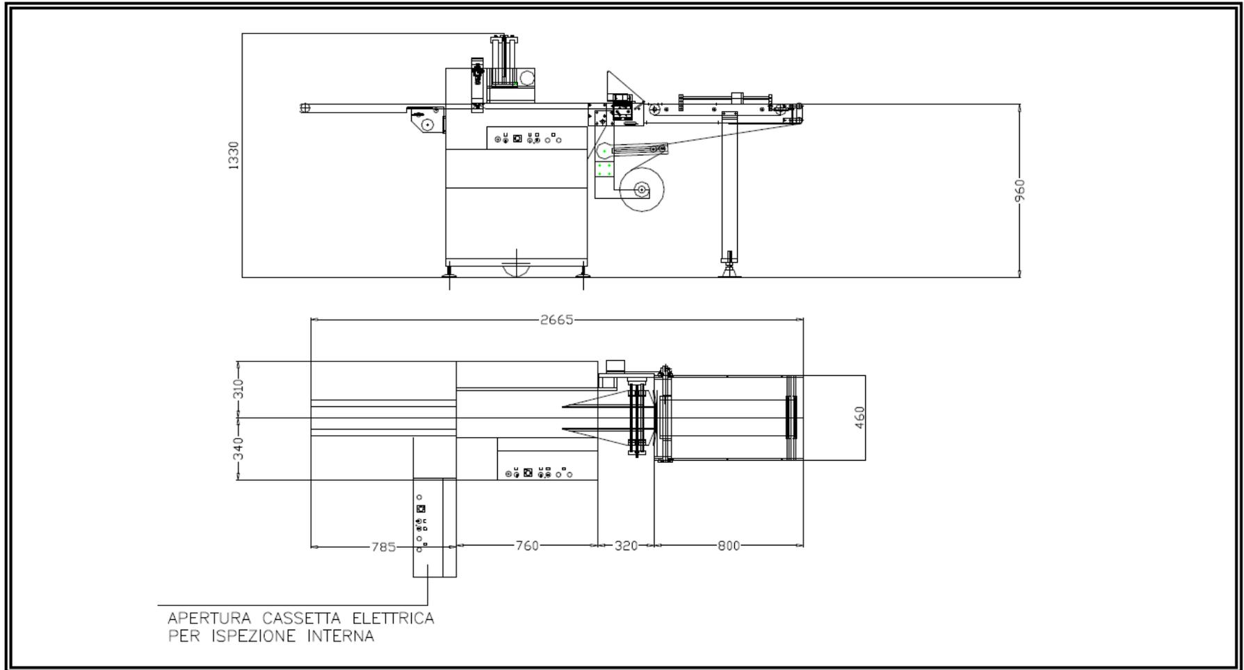
Figure 1 - Configuration standard ensacheuse Micropac Intermittente
